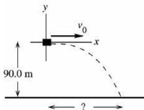
Take the origin of coordinates at the point where the canister is released. Take  $+y$  to be upward. The initial velocity of the canister is the velocity of the plane, 64.0 m/s in the  $+x$ -direction.
