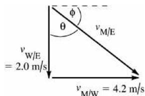
This diagram shows the vector addition  $\vec{v}_{M/E} = \vec{v}_{M/W} + \vec{v}_{W/E}$  and also has  $\vec{v}_{M/W}$  and  $\vec{v}_{W/E}$  in their specified directions. Note that the vector diagram forms a right triangle.
